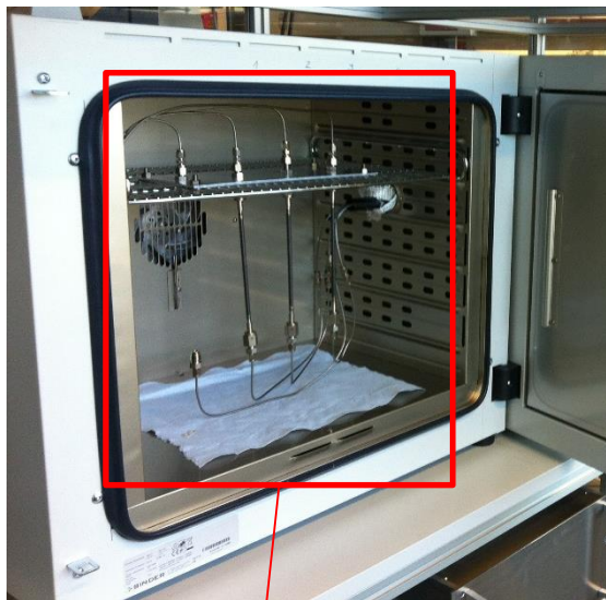
Quadruple fixed bed reactor Size: 0.1 - 0.25 mL Catalyst Volume
