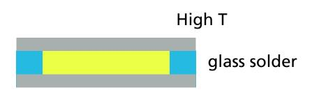
1. Encapsulating "inorganic part" by thermal glass fusing
