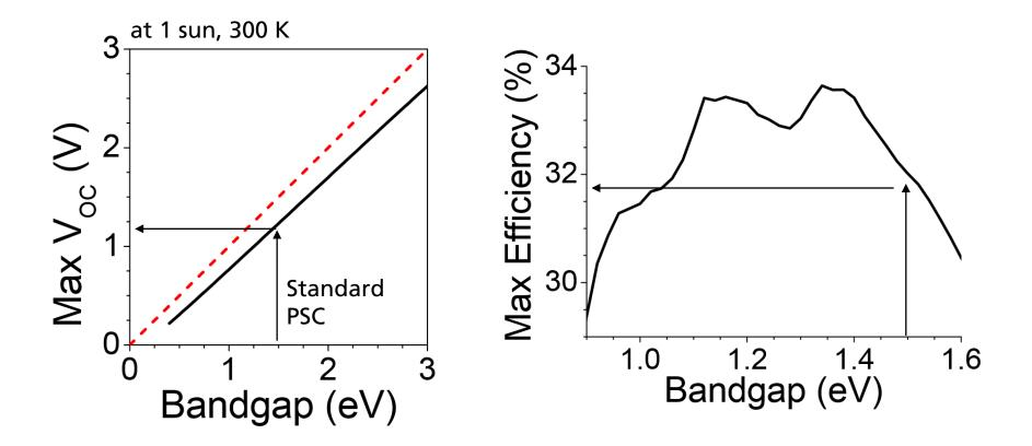
Perovskite solar cells (laboratory) today, V<sub>oc</sub> = 1.0 – 1.2 V, eta = 20 - 22%
