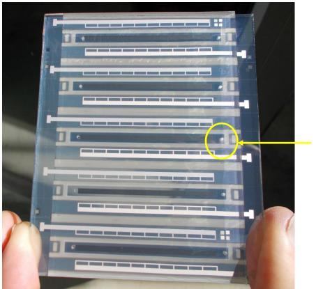
after fusing, before filling with perovskite 1 step solution
