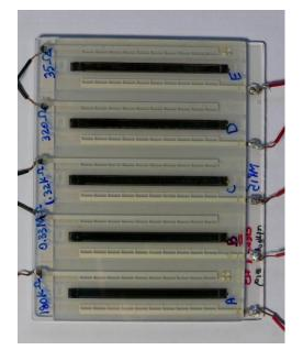
complete cells after annealing under low pressure
